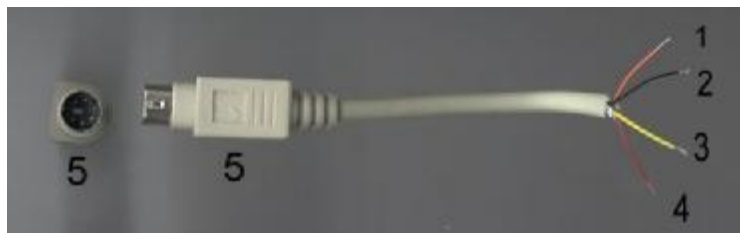
Figure 5: Male PS/2 plug pinouts, connects to target PIC
